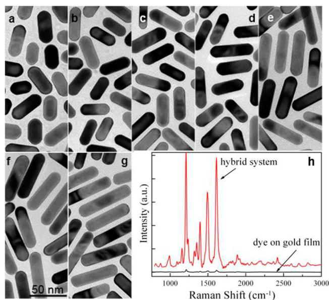
**Figure 1.** (a–g) TEM images of gold nanorods with different aspect ratios and (h) representative surface-enhanced Raman spectrum of the hybrid nanostructure of gold nanorods (sample c) and the J-aggregates of JC-1 dye (red line) in comparison with Raman spectrum of JC-1 dye on a gold film (black line). The PL background was subtracted in both spectra in panel h. The scale bar in panel f is valid for all samples (a–g).
