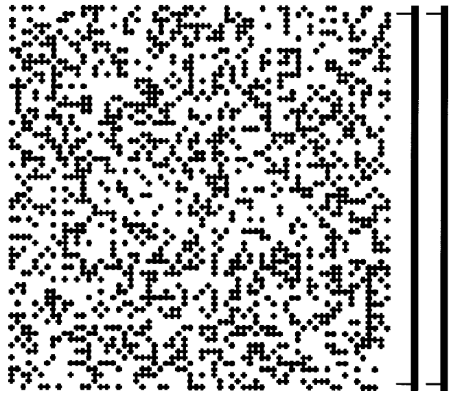
Fig. 2. A picture of the layout with conducting particles for concentration p=0.35 . Some clusters begin to appear. The two lines on the right side are used to normalize the value of the resistance.
