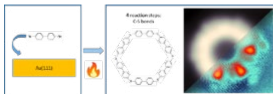
Figure: Schematic representation of the thermally induced thioetherification process of 4'-Bromo-4-mercaptobiphenyl (Br-MBP) molecules on the Au (111) surface. The presence of S atoms strongly modulates the electronic properties of the phenyl chain.
