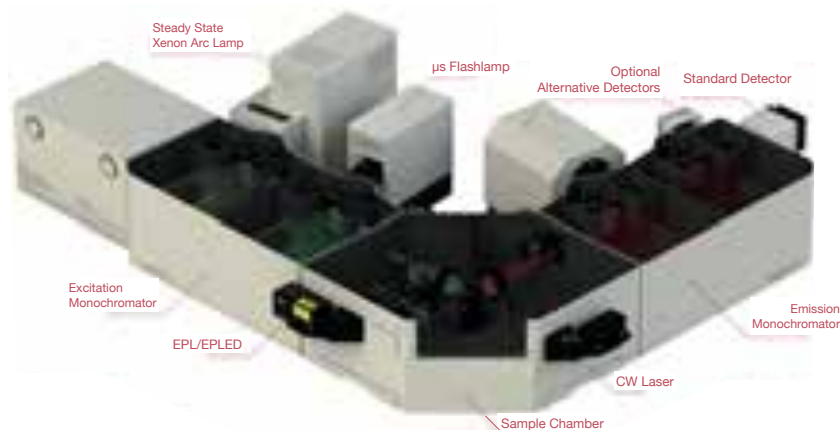
Figure A2.2. Scheme of the fluorescence spectrophotometer used to acquire emission spectra. The main subelements are labelled. EPL/EPLED: Edinburgh Pulsed Laser/LED. CW Laser: Continuous Wave Laser. Taken from [147].
