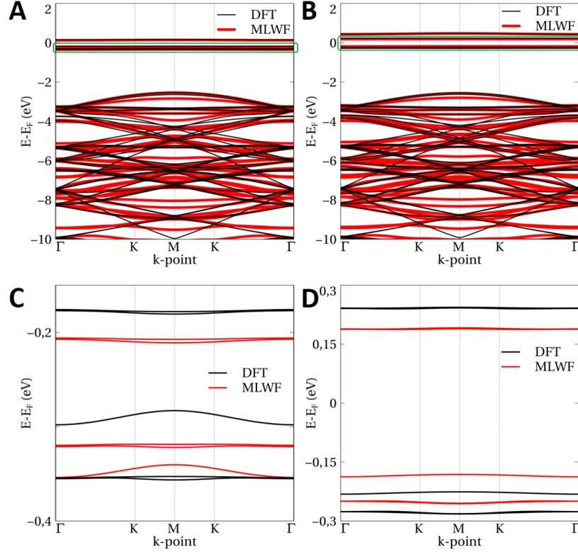
Figure A.1: Bandstructure of Co on h-BN monolayer for a  $4 \times 4$  supercell from DFT (black lines) and MLWF (red lines) calculations. Left panel (A) corresponds to the atop N adsorption site, while the right panel (B) corresponds to the hollow site. (C) and (D) show the energy range in the green squares where Co  $d$  states are located.
