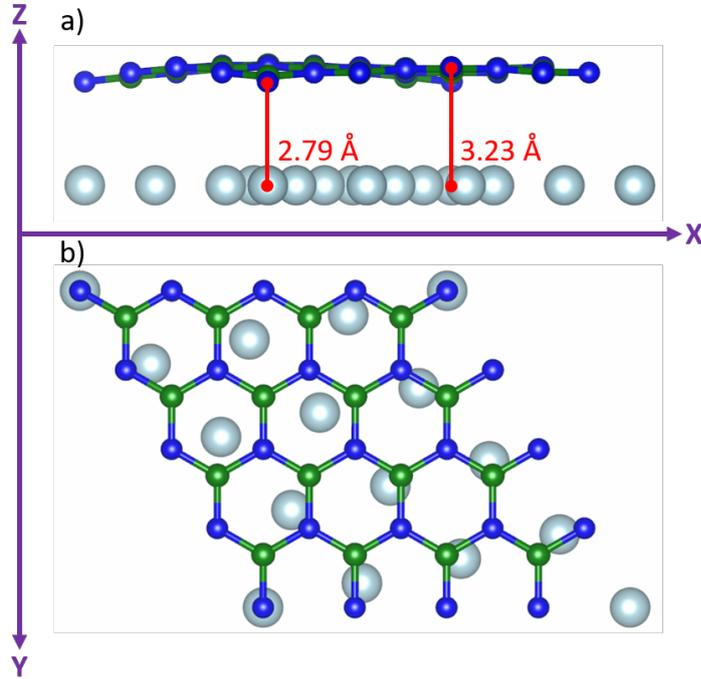
Figure 4.5: a) Side and b) top views of the  $4 \times 4$  supercell for h-BN on Ir(111) surface, after relaxation of the h-BN monolayer in the Z direction. Green and blue spheres represent B and N atoms, respectively, while light blue are the top most layer Ir(111) surface atoms. The side view, a), show a small corrugation of the h-BN on Ir(111) of  $0.44 \text{ \AA}$ .
