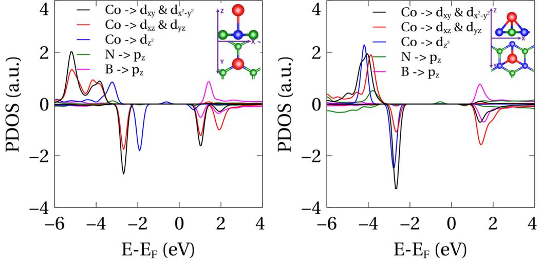
Figure 3.5: Projected density of states (PDOS) onto  $3d$  orbitals of Co and  $p_z$  orbitals of first neighbour N and B atoms for atop N (left) and for hollow (right) adsorption sites, as obtained from the spin-polarized calculations. Positive values correspond to majority-spin and negative values to minority-spin. The insets show the adsorption site, where the red spheres represent the Co adatom, while blue and green spheres represent N and B atoms, respectively.
