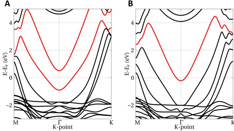
Figure 5.5: Calculated band structure of Au(111) 4 layer slab using the  $1 \times 1$  unit cell. (A) Symmetric slab and (B) slab passivated with H atoms on the bottom. Red bands correspond to the surface state.
