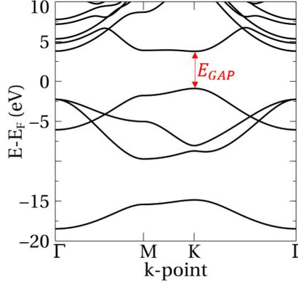
Figure 3.3: Calculated bandstructure of the isolated h-BN.
