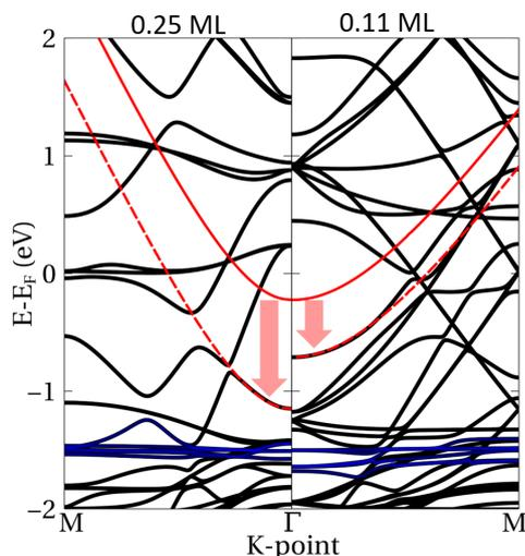
Figure 5.9: Au(111) 4 layer slab band structure for two different Au coverages. The color code is the same as in fig. 5.7, except for blue lines that correspond to Au  $d$ -bands. The left panel corresponds to a coverage of 0.25 ML of Au and the right panel to 0.11 ML. Au adatom  $d$ -bands, in blue, are below the surface state, far from the Fermi energy.
