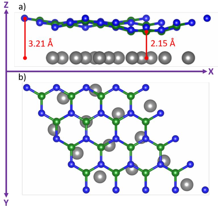
Figure 4.6: a) Side and b) top views of the  $4 \times 4$  supercell for h-BN on the Ru(0001) surface after relaxation of the h-BN monolayer in the Z direction. Green spheres represent B atoms, blue ones N atoms and grey ones the top most layer Ru(0001) surface atoms. The side view show a) shows the high corrugation of the h-BN on Ru(0001) of  $1.06 \text{ \AA}$ .
