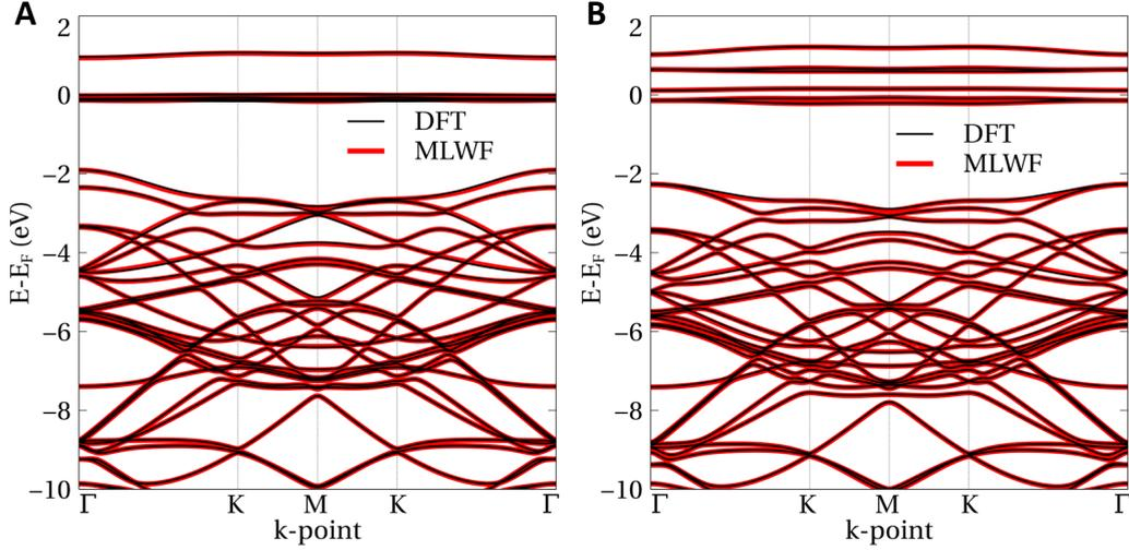
Figure 3.6: Bandstructures of Co on a  $3 \times 3$  monolayer of h-BN obtained from DFT and MLWF calculations. Black lines represent DFT bandstructure and red ones MLWF. Left panel (A) shows the bandstructures for atop N adsorption site and right panel (B) for hollow site.
