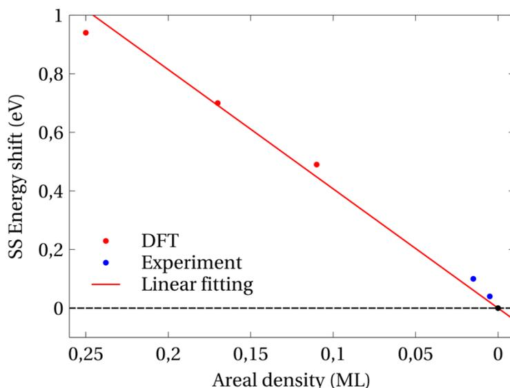
Figure 5.13: Energy shift of the Au(111) surface state due to the Co adatom concentration. Red dots correspond to values obtained from DFT calculations while blue dots were experimentally measured. Red line is the linear fitting of DFT values. The linear fitting is giving quite good agreement between the experimental and theoretical values of the surface state energy shift.
