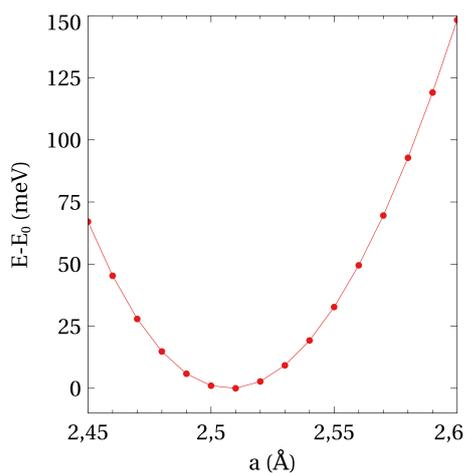
Figure 3.2: Calculation of the optimal lattice parameter. We refer the total energy to the energy of the minimum energy  $E_0$ , which corresponds to the lattice parameter  $a = 2.51\text{ \AA}$ .
