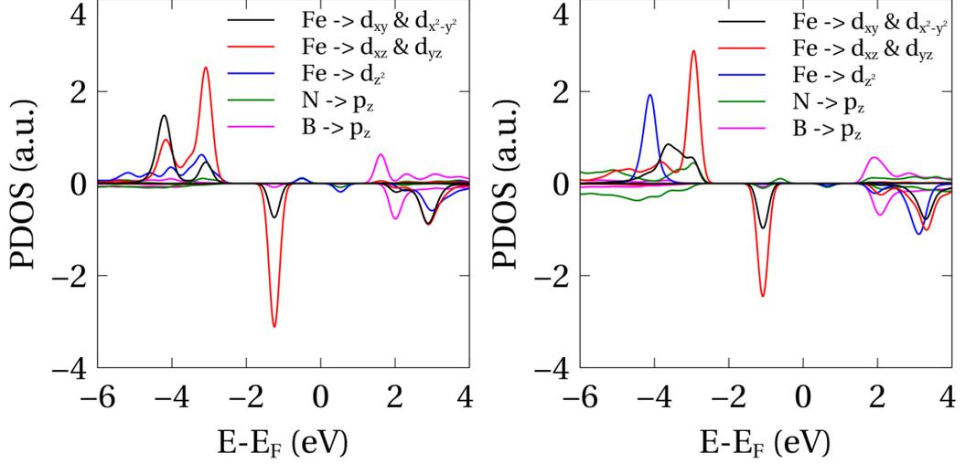
Figure B.1: Projected density of states (PDOS) onto  $3d$  orbitals of Fe and  $p_z$  orbitals of first neighbour N and B atoms once for atop N (left) and once for hollow (right) adsorption sites, as obtained from the spin-polarized calculations. Positive values correspond to majority-spin and negative values to minority-spin.
