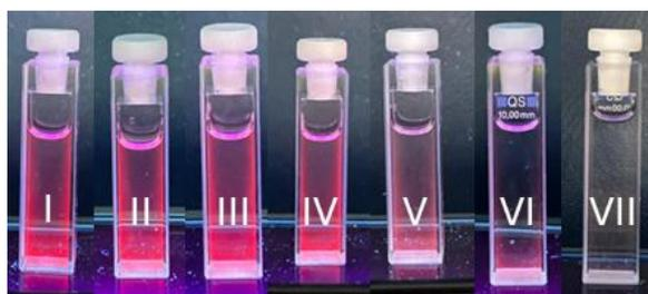
**Figure 13.** (e) demonstration of the utility of Eu-SCNPs as “visual” pass/fail sensors of m.p.c. of Cu<sup>2+</sup> ions in water according to the WHO criterion (i: 5 μM, ii: 10 μM, iii: 15 μM, iv: 22.5 μM, v: 25 μM, vi: 27.5 μM and vii: 30 μM).
