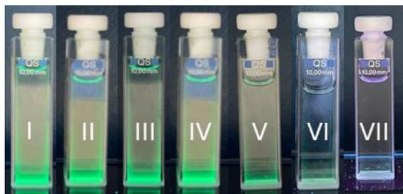
**Figure 17.** demonstration of the utility of Tb-SCNPs as “visual” pass/fail sensors of m.p.c. of Cu<sup>2+</sup> ions in water according to the WHO criterion (i: 2.5 μM, ii: 5 μM, iii: 15 μM, iv: 22.5 μM, v: 25 μM, vi: 27.5 μM and vii: 30 μM).
