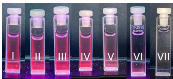
Figure 13. (e) demonstration of the utility of Eu-SCNPs as “visual” pass/fail sensors of m.p.c. of Cu 2+ ions in water according to the WHO criterion (i: 5 μM, ii: 10 μM, iii: 15 μM, iv: 22.5 μM, v: 25 μM, vi: 27.5 μM and vii: 30 μM).
