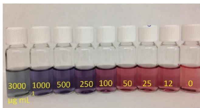
Figure 13. Photographs of the sensing system in the presence of decreasing concentrations of zein.<sup>89</sup>
