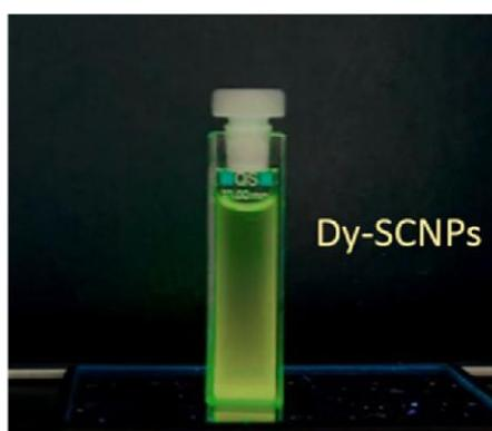
**Figure 33.** Illustration of the yellowish fluorescent Dy-SCNPs under UV light irradiation ( $\lambda_{exc} = 254$  nm) .
