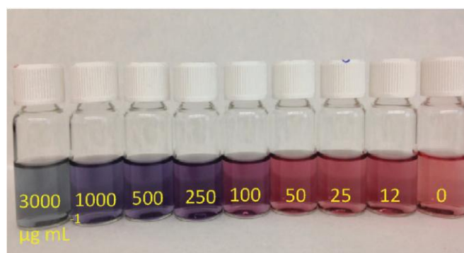
Figure 13. Photographs of the sensing system in the presence of decreasing concentrations of zein. 89
