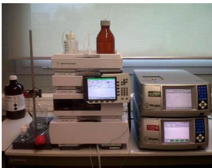
Figure 2.1. GPC equipment used in this work.
