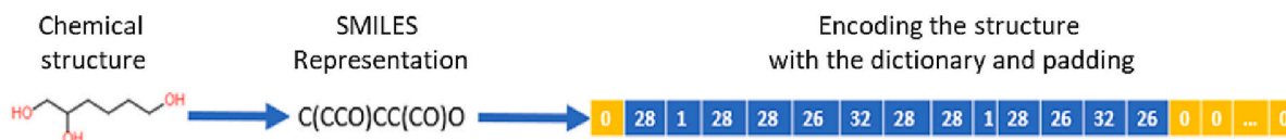
Fig. 1. Encoding the SMILES with cardinal encoding. We added a 0 at the beginning of each string and completed them with a padding of 0s to have the same length for all the instances.
