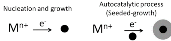
Figure 1.4: Main mechanisms for the synthesis of AuNPs. In the nucleation and growth mechanism, a strong reducing agent reduces metal ions followed by growth into nanoparticles. In the seeded-growth process, the reduction of metal ions takes place exclusively on the surface of preformed seeds to produce particles of the desired shape and size. Reproduced from [20]
